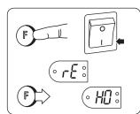
Hold in the (F) key and then switch the heater ON.
