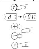
Press ⑦ for 5 seconds. d (days) will flash 3 times. 01 (days) will flash continuously.
