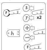
Hold down on  $\bigcirc$  and press twice on  $\bigcirc$  or  $\bigcirc$ . Release F and h (hours) will flash 3 times.
