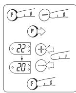
Hold down on F and press once on Release F. °C will flash 3 times and the setpoint temperature will flash. Press + or until the display shows the same as the actual measured room temperature. Store by pressing F for seconds.
