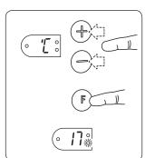
°C will flash three times and then 17 (°C) will flash continuously. With the ⊕ or ⊝ key select your preferred cutback temperature.
