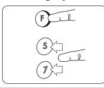
Hold down (F) and press once on (T) or (S) to override the current active period, or the next period of temperature cutback. The lamp is lit steadily for the period in question. Temperature cutback will resume as usual from the subsequent period.
