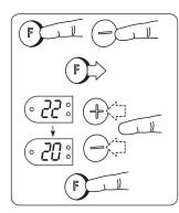
Hold down on **(F)** and press once on **(⊃)** Release **(F)**. °C will flash 3 times and the setpoint temperature will flash. Press **(+)** or **(□)** until the display shows the same as the actual measured room temperature. Store by pressing **(F)** for 5 seconds.
