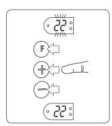
At the time the frost-safe period ends, the comfort temperature setting will flash to indicate the need for action.
