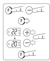
Hold down on F and press once on C Release F. C will flash 3 times and the setpoint temperature will flash. Press + or until the display shows the same as the actual measured room temperature. Store by pressing F for seconds.
